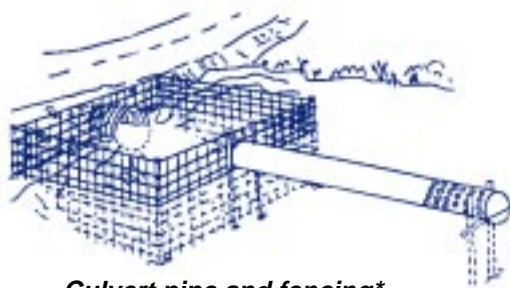
Culvert pipe and fencing*
